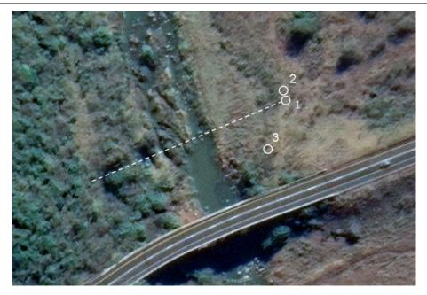
Figure H3 Location of the surveyed cross-section at the downstream end of a boulder rapid; approximate positions of bench marks/fixed stations are indicated with circular markers; flow direction is top-to-bottom
